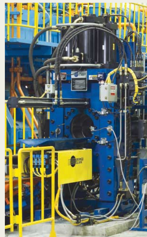
The Granco Clark Log Shear allows you to reduce both inventory and scrap because it cuts billets to the correct length as needed.
