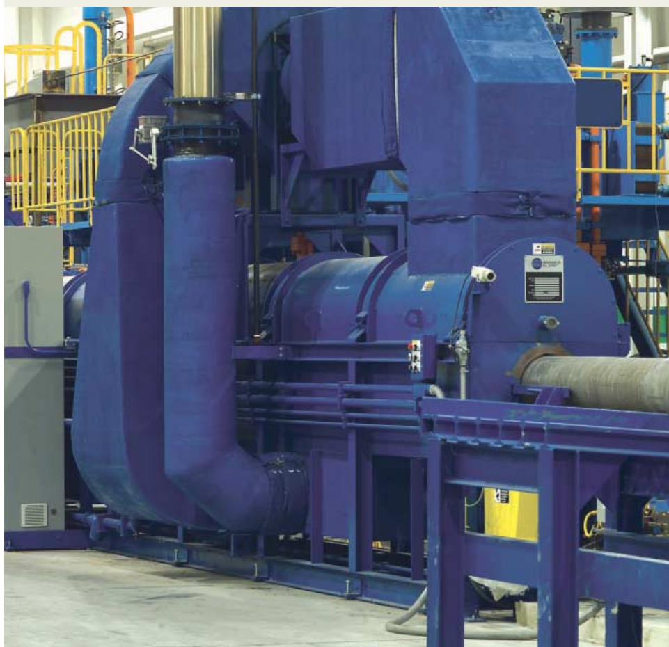
A “hot jet” preheat section boosts thermal efficiency.
