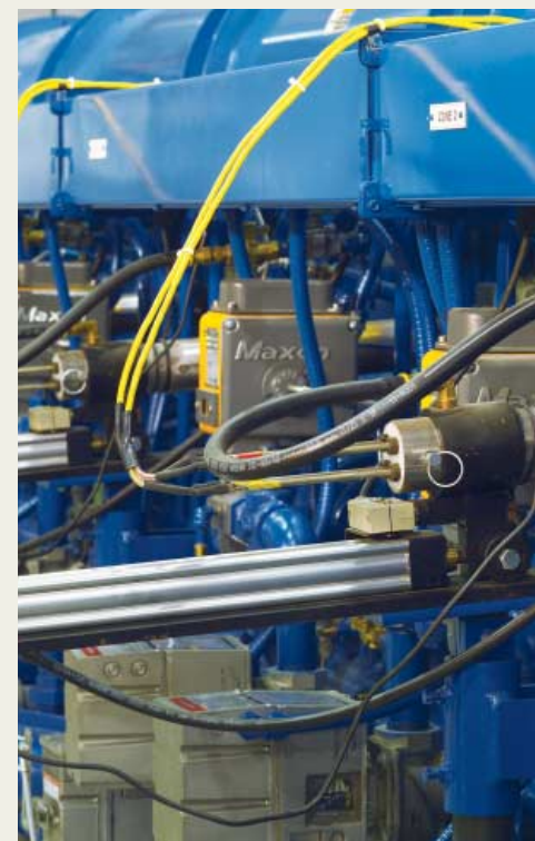
Multiple thermocouple probes monitor the heating zones to assure precise, consistent temperatures.
